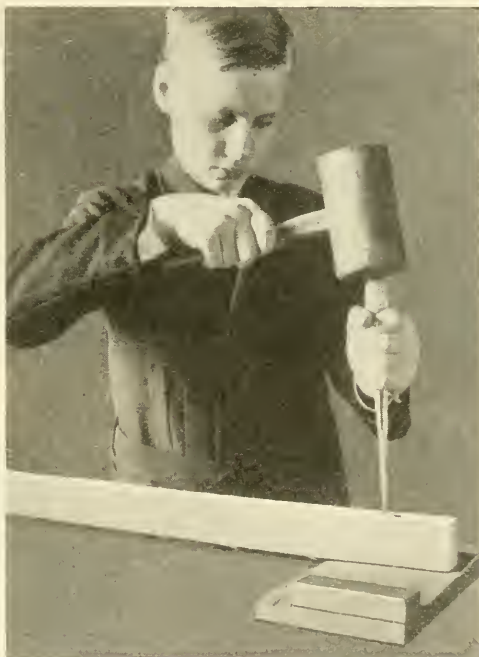
Fig. 19. Position of Chisel and Mallet for Mortising.
